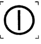
A circle with a vertical bar inside is centered within a square frame. The frame has L-shaped corner brackets at the top-left and bottom-right corners. | 接通和断开                             | 5010        |
